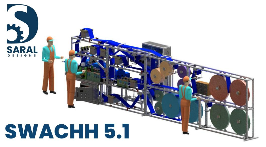
Automatic High speed machine for making premium quality sanitary pads
