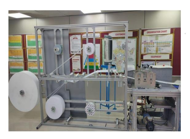
**Swachh 7.0** is a fully-automatic machine for producing 3 ply surgical masks.
