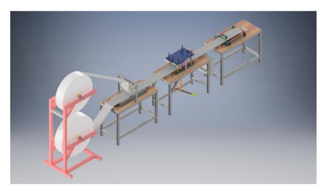
Swachh Micro is a Manual Sanitary Napkin making machine for producing high quality ultrathin sanitary napkins.
